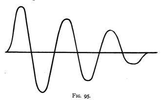
When the resistance of the discharge circuit exceeds a certain value the charge will not oscillate. This critical value has been reached when R is greater that  $2\sqrt{\frac{L}{C}}$ . When the capacity, inductance and resistance are known the frequency can be obtained by the equation
