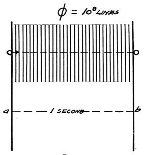
If the conductor moves at a uniform rate of speed from **a** to **b** in one second, it cuts lines at every instant at the rate of  $10^8$  lines per second, which generates an e. m. f. of 1 volt. In this case the maximum and average voltage are the same, as is shown in Fig. 60.
