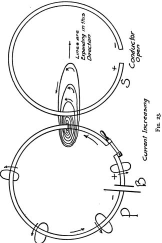
as the first, the lines of force must pass through it during their expansion, as shown in Fig. 23.
