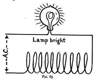
incandescent lamp. The lamp burns at almost full candle-power, as the inductance of the coil is very small.
