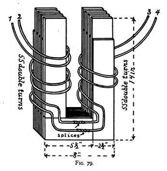
using 1 and 4 for terminals. For parallel connection 1 and 2 are switched together as one terminal, while 3 and 4 are switched together for the other terminal. The upper ends of the wire should be left standing straight up so that the secondary coils may be easily slipped down over the primary winding without injury.
