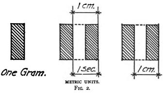
The force of gravity is 981.45 centimeters per second; therefore, the force required to **oppose** it in lifting one gram, one centimeter high, is 981.45 dynes. Thus the dyne can be expressed in weight, or 1-981.45 gramme.
