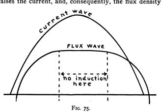
and if the voltage gets too high the core becomes saturated before the current in the primary has reached its maximum. The result is that the top of the flux wave becomes perfectly flat, as shown in Fig. 75.
