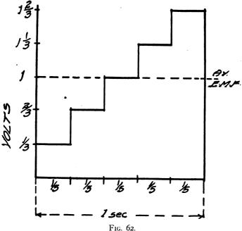
When the movement is nearly at right angles to the flux, the e.m. f. is, of course, higher than in Fig. 60.
