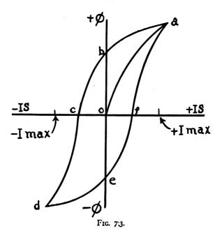
m. m. f. from f to maximum creates the flux from f to a. The flux never again increases as it did from o to a, because of the residual magnetism in the iron. Every succeeding cycle of flux changes from a to b, c, d, e, f and a.
